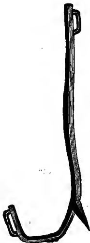
FIG. 228.—Eastern pole climbers, with and without strap for attaching to legs.
